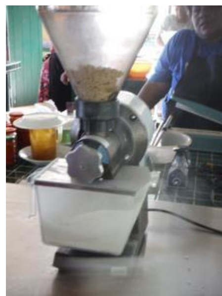
Grinder to manufacture four manufactured four by PIFON used for breadfruit
